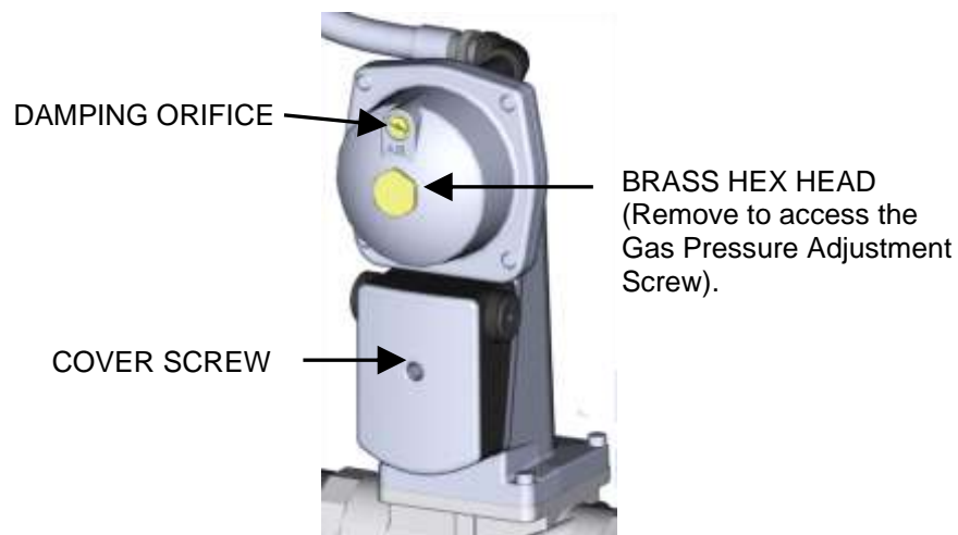
Figure 5-3: SSOV Actuator With Gas Pressure Adjustment (SKP25)
