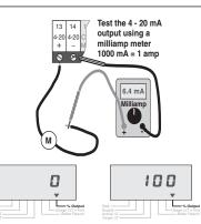
Reading should be 4 mA Reading should be 20 mA
