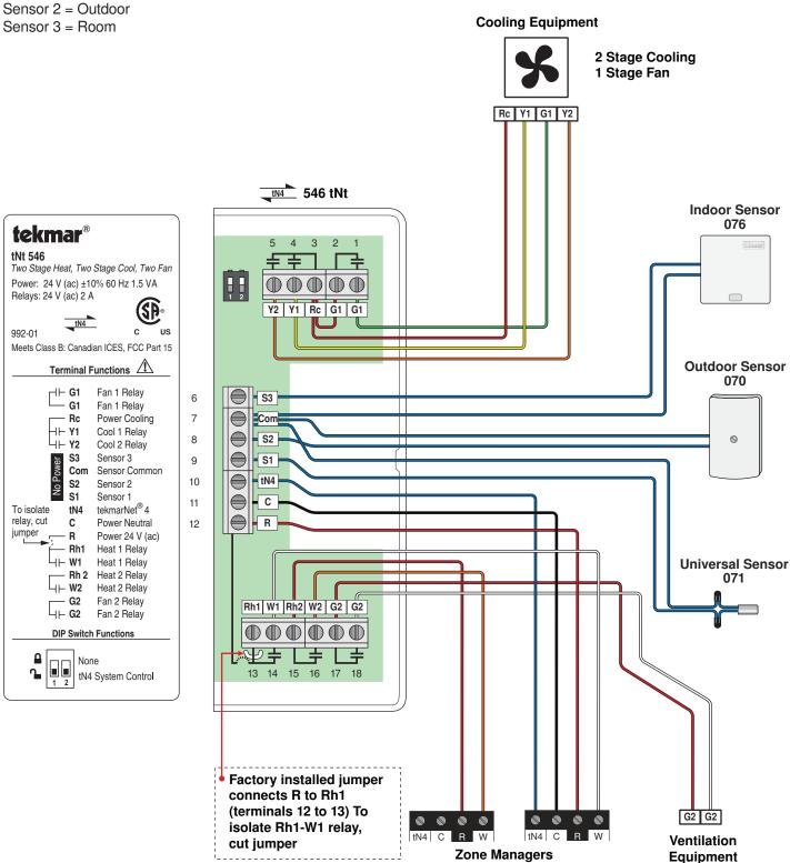
Two Stage Heating (H1 = Fin-tube Convector, H2 = Furnace), Two Stage Cooling (C1 = Compressor 1st stage, C2 = Compressor 2nd stage), Two Speed Fan (F1 = Low-H2 & C1, F2 = High-C2), Fan Mode = 5.
