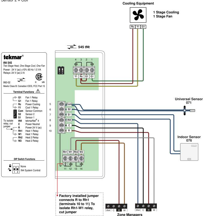
Two Stage Heating (H1=Radiant, H2=Furnace), One Stage Cooling (C1=Compressor), One HVAC Fan (F1=H2 & C1), Fan Mode=2.
