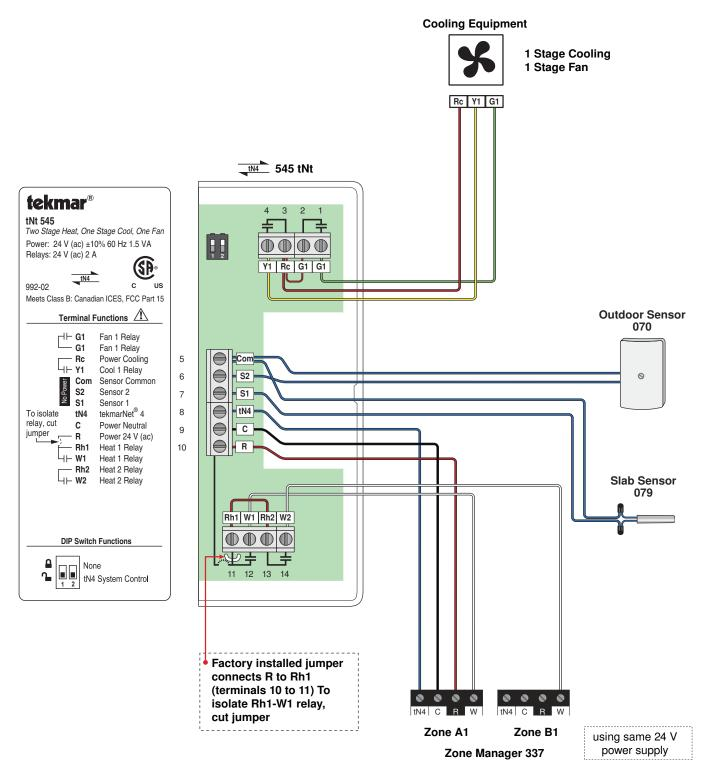
Two Stage Heating (H1=Radiant, H2=Fan Coil), One Stage Cooling (C1=Compressor), One HVAC Fan (F1=H2 & C1), Fan Mode=2.
