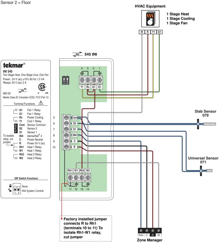
Two Stage Heating (H1=Radiant, H2=Fin-tube Convector), One Stage Cooling (C1=Compressor), One Ventilation Fan (F1=HRV or Vent), Fan Mode=None.
