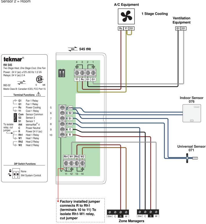
Two Stage Heating (H1=Fan Coil, H2=Furnace), One Stage Cooling (C1=Compressor), One HVAC Fan (F1=H1 & H2, C1), Fan Mode=2.
