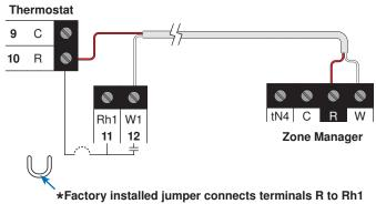
(To isolate Rh1-W1 relay, cut jumper)
