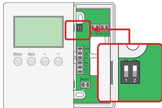
**Note:** The tN4 System Control's Lock/Unlock DIP switch overrides the Lock/Unlock DIP switch on the 544. Set the tN4 System Control's Lock/Unlock DIP switch to the Unlock position before Access Levels can be changed on the thermostat.
