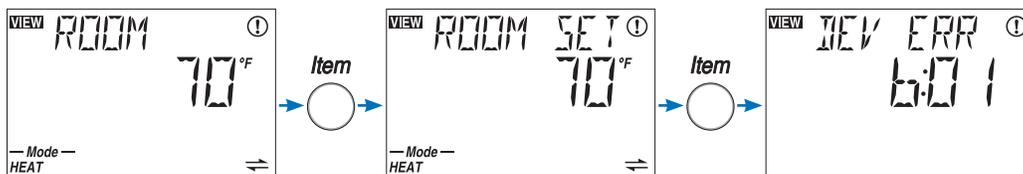
If the error message is a Device Error (if “DEV” or “DEV ERR” is shown on screen), read the address shown and go to the device with that address. That device will have a Local Error indicating specifically what the problem is. When the problem is corrected, the error message will automatically clear.
