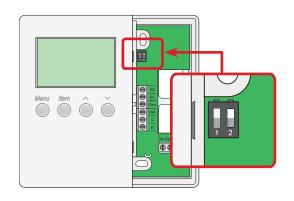
*Note:* The tN4 System Control's Lock/Unlock DIP switch overrides the Lock/Unlock DIP switch on the 543. Set the tN4 System Control's Lock/Unlock DIP switch to the Unlock position before Access Levels can be changed on the thermostat.
