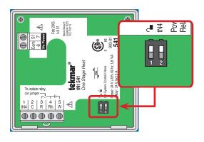
**Note:** The tN4 System Control's Lock/Unlock DIP switch overrides the Lock/Unlock DIP switch on the 541. Set the tN4 System Control's Lock/Unlock DIP switch to the Unlock position before Access Levels can be changed on the thermostat.
