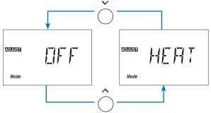
If no schedule is being used, the heating temperature can be permanently adjusted from the View menu when viewing either the "Room" or "Room Set" items.
