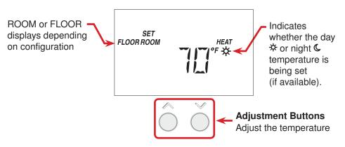
You will be adjusting the temperature of the current operating mode. To adjust temperature settings that are not shown on the screen, you must enter into the Adjust Menu as described in the "Adjust Menu" section. There may be other symbols on the screen that affect thermostat operation. Please see the "Display Symbols" section for a description of each symbol.
