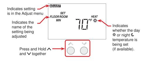
This thermostat has access levels. It will typically be installed and programmed by a heating professional and then locked in a "User" access level. System critical settings will not be available for adjustment. For more information on these settings, please consult your installing contractor or this product's Installation and Operation Manual. The following pages describe the settings available to the "User".
