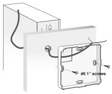
**NOTE:** If the thermostat is to be used for remote sensing (i.e. The built-in air sensor is disabled and an indoor sensor is being used.) Mount the thermostat in the desired location in an appropriate manner.
