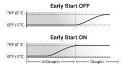
**Cooling** - The early start function, when used with cooling, allows the cooling system to turn on 30 minutes prior to the beginning of a period that requires cooling.
