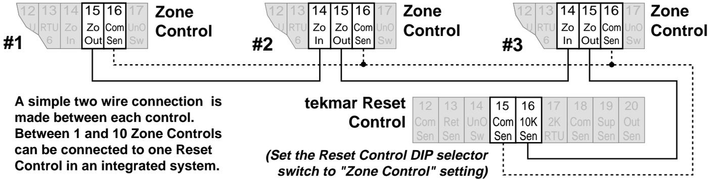
A simple two wire connection is made between each control. Between 1 and 10 Zone Controls can be connected to one Reset Control in an integrated system.
