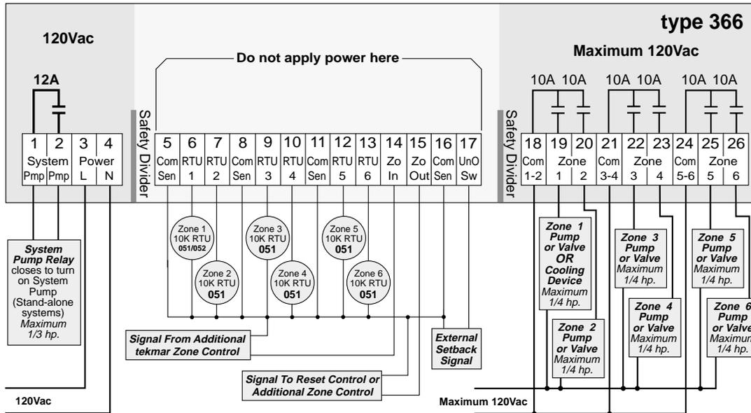
**Note: This illustration shows the various devices that can connect to the 366, and is not a wiring diagram. For a detailed wiring schematic of your specific application, refer to the Application Brochure A 366.**
