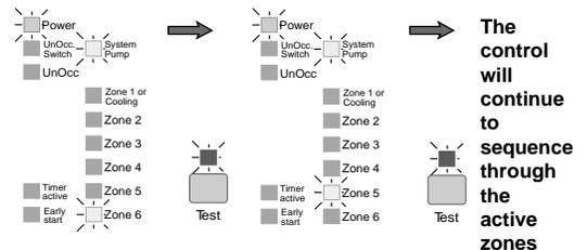
If the Test Button is pushed once during the time a zone is open, the "Test" light will flash and the control will be held in a pause mode for 5 minutes, after which time it will automatically exit the test routine and return to normal operating mode. Pushing the Test button during the 5 minute pause will allow the control to resume the test routine at the next step.
