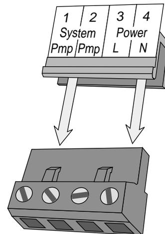
Terminal plug disconnected from its header on the control
