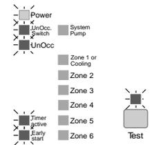
*Note: Whenever the control exits the test routine, there is an automatic 3 second delay before the control will allow re-entry. Pushing the test button during this 3 seconds will have no effect.*
