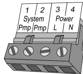
Terminal plug pushed into its header on the control
