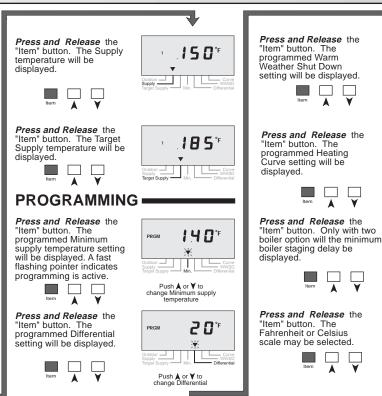
The control automatically goes back to viewing when the buttons are left alone for 20 seconds -
