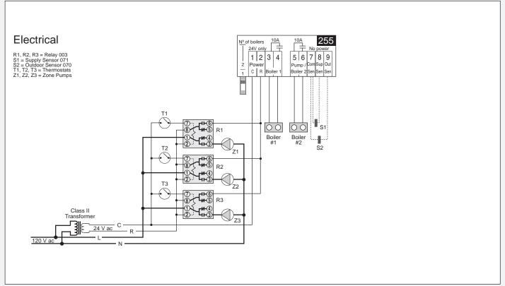
**Note:** This is only a concept drawing. The designer must determine whether this system will work in his system and must ensure compliance with code requirements. Necessary auxiliary equipment, isolation relays (for loads greater than the specified tekmar internal relay ratings), and other safety and limit devices must be added.
