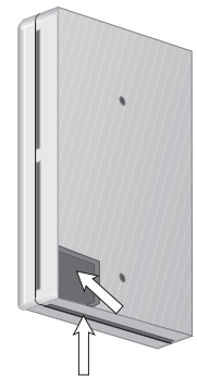
Wiring can enter through the back or the bottom of the enclosure.
