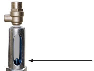
Figure 2 Position Indicator Stem in Down Position Indicating Valve Closed
