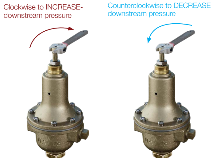
Figure 2 CP15 — Pressure Reducing Control
