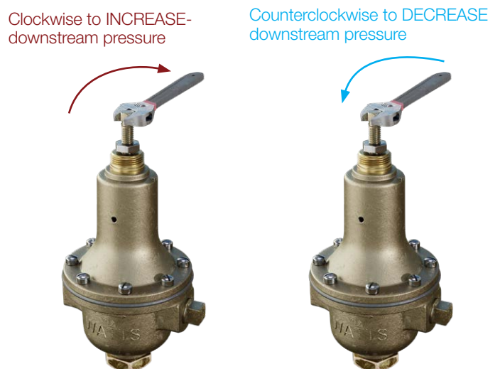
Figure 2 CP15 — Pressure Reducing Control
