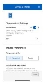
The Device Settings page for specifying the temperature units and the Heat to Away setpoint when the Setpoint Control is in heat mode.
