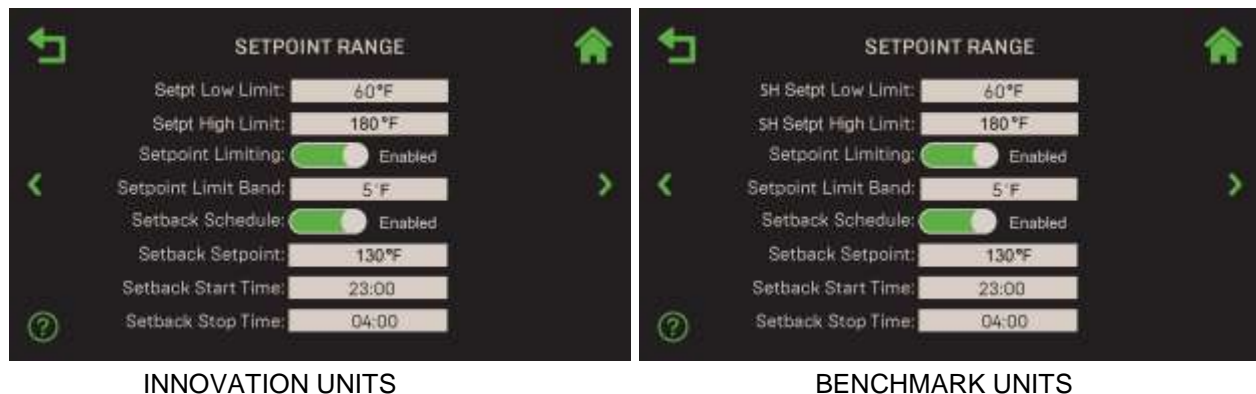
Figure 4.6.1.3: Operating Controls: Setpoint Range Screen
