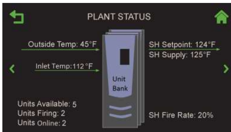
Figure 5.3: Plant Status Screen – Benchmark Only
