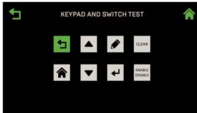
Figure 3.2-4: Diagnostics: Keypad and Switch Test Screen
