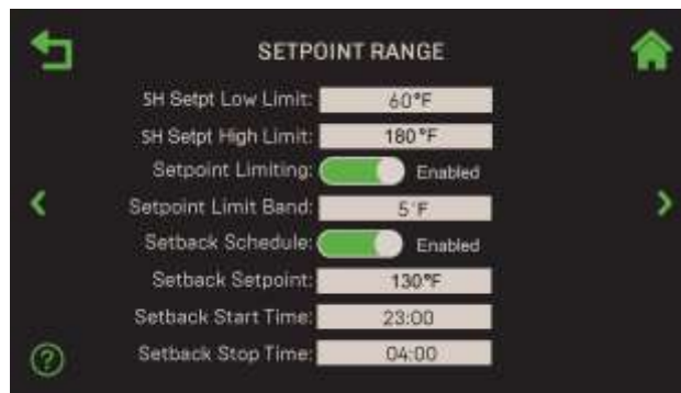
Figure 4.3.4.5: Operating Controls: Setpoint Range Screen
