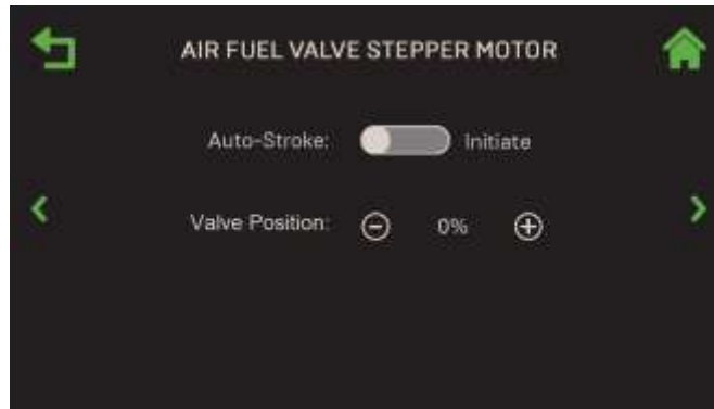
Figure 3.4.1-1: Subsystems: Air Fuel Valve Stepper Motor Test Screen
