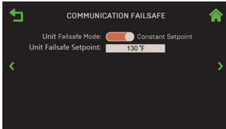
Figure 4.4.4: Comm & Network : Communication Failsafe Screen
