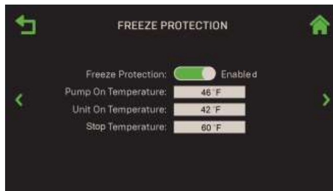
Figure 4.2.5: Unit : Freeze Protection Screen – Freeze Protection Enabled
