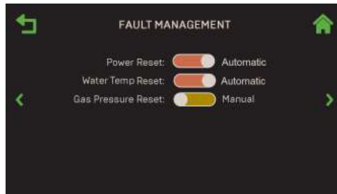
Figure 4.2.4: Unit : Fault Management Screen
