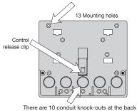
and bottom of the wiring chamber.
