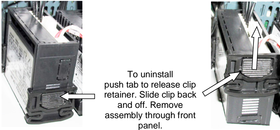
Figure 8-8b. Over-Temperature Switch & Temperature Indicator Installation
