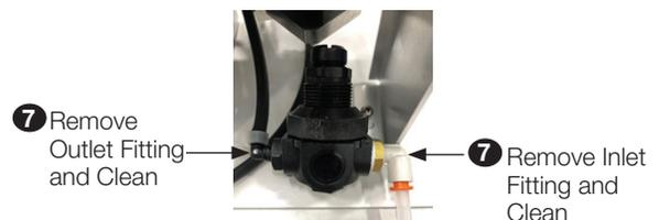
8. Clean off the old fittings and apply new Telson tape to the threads of the fittings.
