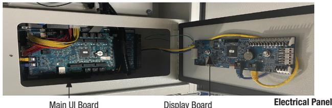
All electrical connections are located in the upper electrical compartment. The electrical compartment access at the front can and should only be opened during installation. No power should be applied until the electrical compartment access is closed and sealed.
