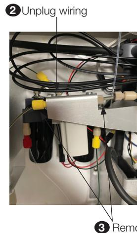
3. Remove fittings from solenoid valve inlet and outlet.
