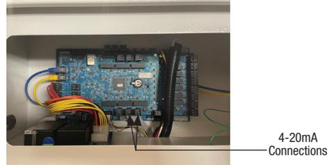
Main UI Board Located inside the Electrical Panel
