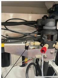
5. Using a screwdriver, loosen the screw on the optical assembly that holds the reagent injectors in place.
