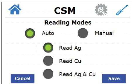
4. Once the desired Reading Mode has been saved, press the
