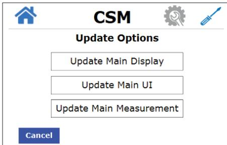
4. After pressing the update option, the firmware will begin to update. A status update will appear on the screen to display the progress of the update. Once the update is complete, a restart of the instrument is required.
