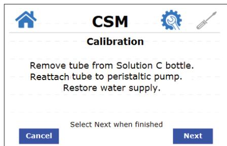
Calibration is now complete. Calibration data is saved after all steps are complete. If calibration is canceled at any point in the calibration process, the last successful calibration data remains stored. The CSM returns to normal operation once calibration is complete.
