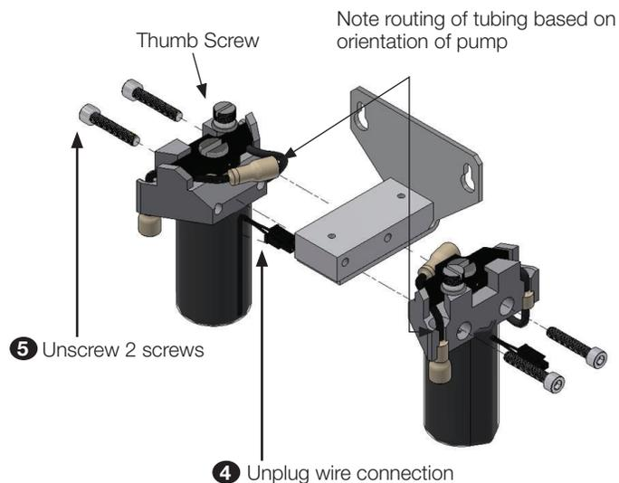
6. Install new reagent pump to the mounting block using the 2 screws removed in Step 5.
