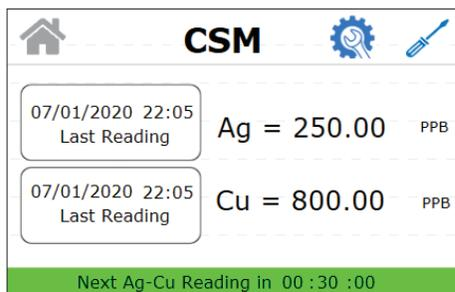
This monitor allows for the measurement of the copper and silver output from a copper silver ionization disinfection system in a water source. Measurements are usually taken in Parts per Billion (ppb). The CSM can measure silver (Ag) dilutions ranging from 50ppb to 250ppb and copper (Cu) dilutions ranging from 200ppb to 2000ppb. Any measurement outside of these ranges will give a screen notice that the measurement is out of range. The reading will be shown but the accuracy can not be guaranteed.
