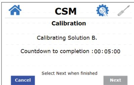
8. Remove tube from Solution B bottle, rinse with Solution D. Insert tube into Solution C bottle (High Range Copper/Silver). Press **Next**.
