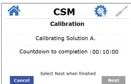
6. Remove tube from Solution A bottle, rinse with Solution D (DI water). Insert tube into Solution B bottle (Mid Range Silver). Press **Next**.
