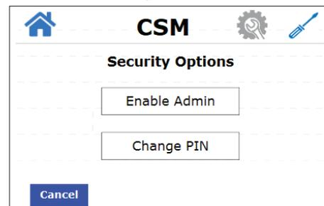
4. If selecting to **Enable Admin**, enter the security PIN again to enable. If selecting **Change PIN**, enter the new pin. You will be prompted to enter the new pin a second time. Then press **Enter**.
