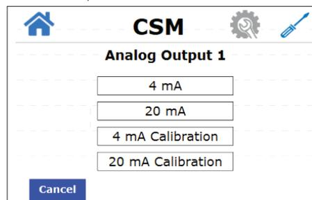
4. Use the up and down arrows to input the desired setting and then press **Save**. Do this for the remaining output settings for Analog Output Ag and Cu, if desired.
