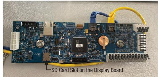
Display Board Located on the Electrical Panel Door
