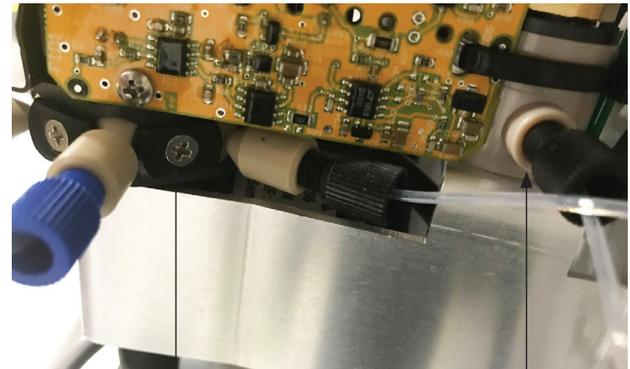
To replace the air pump tubing on the CSM instrument:
