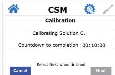
10. Remove tube from Solution C bottle and reattach tube to peristaltic pump. Restore the water supply and click **Next**.
