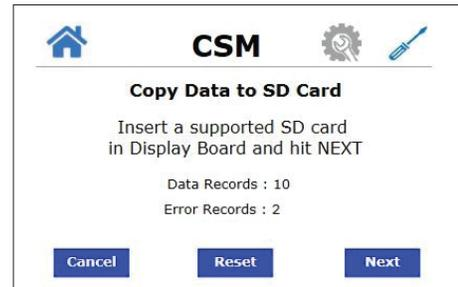
3. After pressing NEXT, the data will be copying to the SD card. A status update will appear on the screen stating Copying Records to SD Card in Progress... Once the data has been copied to the SD card, a completion update will appear on the screen.
