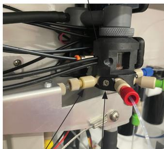
8. Rotate the check valve retainer 90° and disconnect the injector from the optical assembly.
