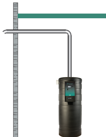
Sealed combustion with sidewall terminations
