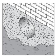
Drill a hole according to minimum and maximum dimensions (see column wall opening).
