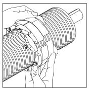
Loosen rear pressure plate with nut just enough so links move freely. Check to be sure all bolt heads are facing the installer. Extra slack or sag is normal.
