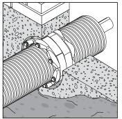
Slide belt assembly into annular space. Start inserting Link-Seal modular seal assembly at the 6 o'clock position and work both sides up toward the 12 o'clock position
