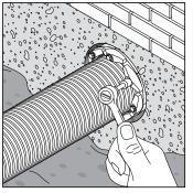
4. Using a hand socket or offset wrench ONLY, start at 12 o'clock. Do not tighten any bolt more than 4 turns at a time. Continue in a clockwise manner until links have been uniformly compressed. (Approx. 2 or 3 rotations)
