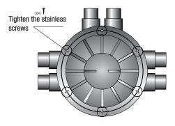
Carefully turn the lid clockwise to lock it. Do not damage the black gasket between body and top part.
