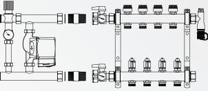
The IsoTherm Mixing Module is a simple, compact, pre-piped pump and mix valve assembly designed to thread directly to a 1" Stainless Steel manifold. Optional BSP x NPT transition nipples are provided with the IsoTherm to allow connection to trunk isolation ball valves.
