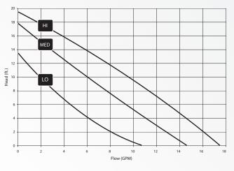
The IsoTherm module uses a Grundfos 3 speed circulator. Flow capacities can be modified by adjusting the speed setting from HI, MED, or LO. Corresponding curve capacities are shown in the graph above.
