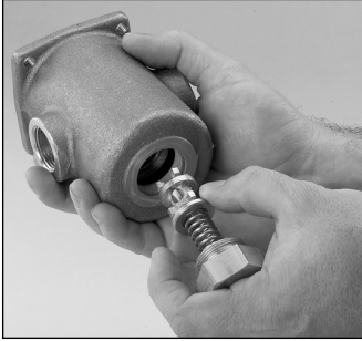
Insert the cold water poppet, spring, and plug into the bottom of the lower housing.
