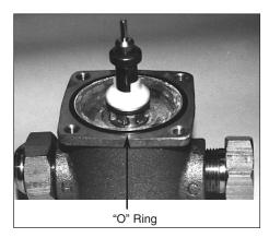
10. Reassemble the motor housing cap/adjustment knob assembly to the motor housing using the new gasket and four (4) screws. Insure the overload assembly is inserted straight in the motor housing and engages the stem of the thermal actuator.
