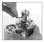
To vary discharge temperature, turn temperature adjustment knob. This knob may be locked in place by inserting a hex key inside opening and turning lock screw clockwise until tight.
