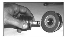
4. Place the "O" ring on the stem of the new overload assembly. Grease the stem of the overload assembly, and insert it into the adjustment knob.
