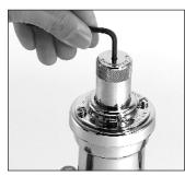
To lower maximum temperature setting, turn adjustment knob to full hot position (counterclockwise). Insert hex key in adjusting screw as shown. Hold adjustment knob and turn adjusting screw until desired maximum temperature is obtained.
