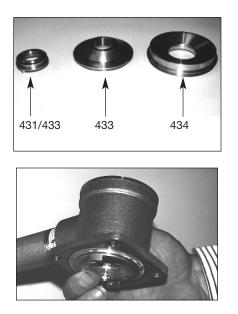
Set the thermal actuator on the motor adapter, and carefully assemble the valve back to the motor housing using the new "O" ring supplied. Tighten the union nuts hand tight, and reinstall the four (4) bolts between the valve assembly and motor housing.
