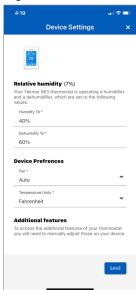
The Device Settings set the temperature units, fan, relative humidity and floor setpoints.
