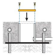
• Fasten the 097 to the socket 091 using the 4 stainless steel screws provided with the Socket 091.
