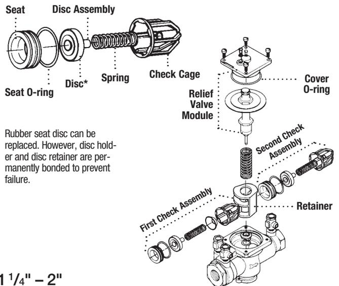
Rubber seat disc can be replaced. However, disc holder and disc retainer are permanently bonded to prevent failure.
