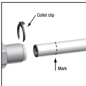
4. Push tubing into tailpiece up to mark.
